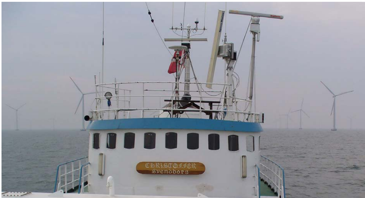
Fig. 2.4: Set up of horizontal and vertical radar on the MS Christoffer
