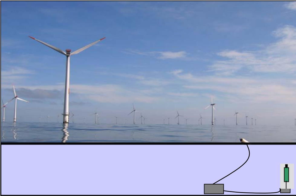
Fig. 2-14: Deployment of a T-POD at sea.
