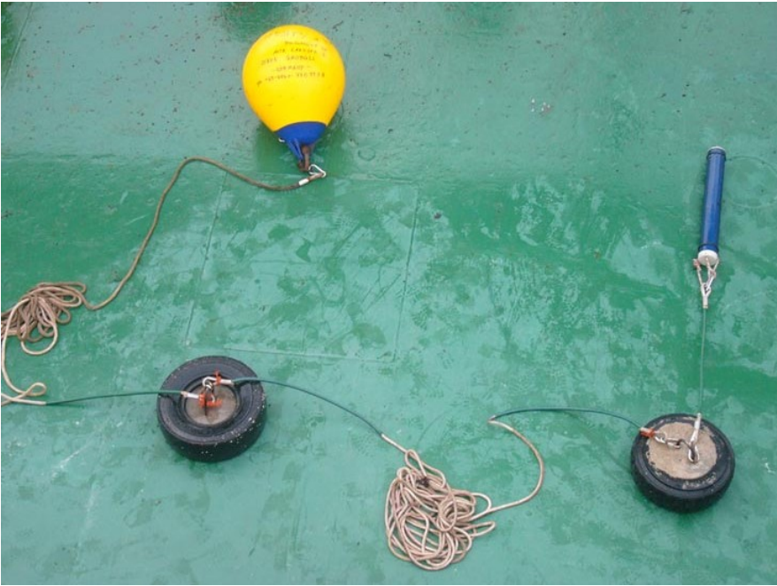
Fig. 2-15: T-POD mooring system with two anchor blocks (tyres with concrete).
