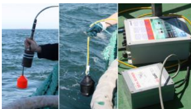
Fig. 1: Left to right: Lofitech transducer with ballast weight attached, Airmar transducer, control units of the two devices.
