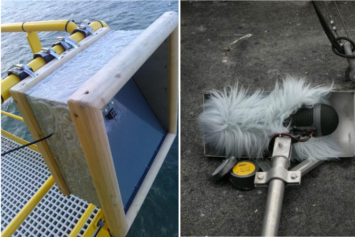
Figure 3.2 Microphone systems used at OSS 'Butendiek' and OSS 'Nordsee Ost' (left) and on FINO1 (right, from OREJAS et al. 2005).
