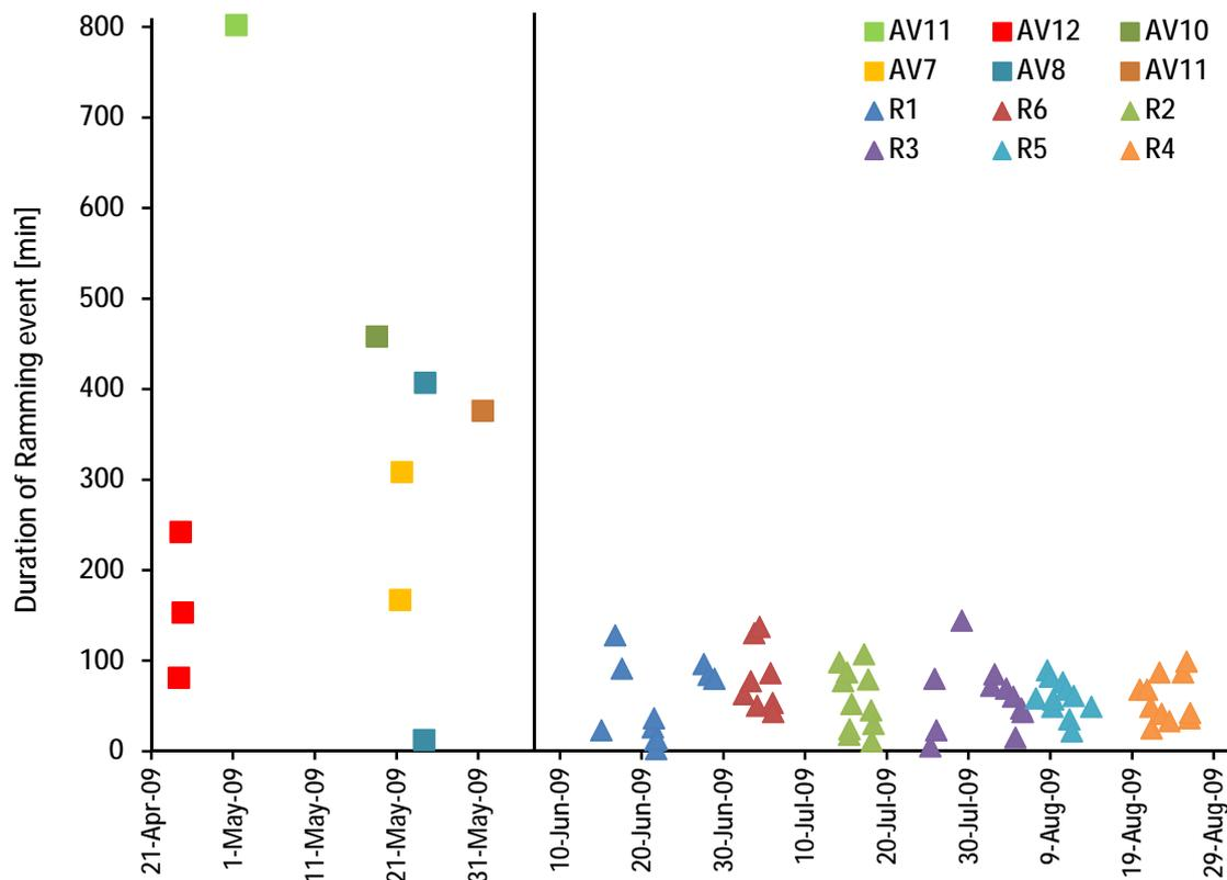
Fig. 2-4: Date and duration of Pile-driving events for the offshore windfarm alpha ventus; vertical line separates Tripod (left) from Jacket (right) Pile-driving events.
