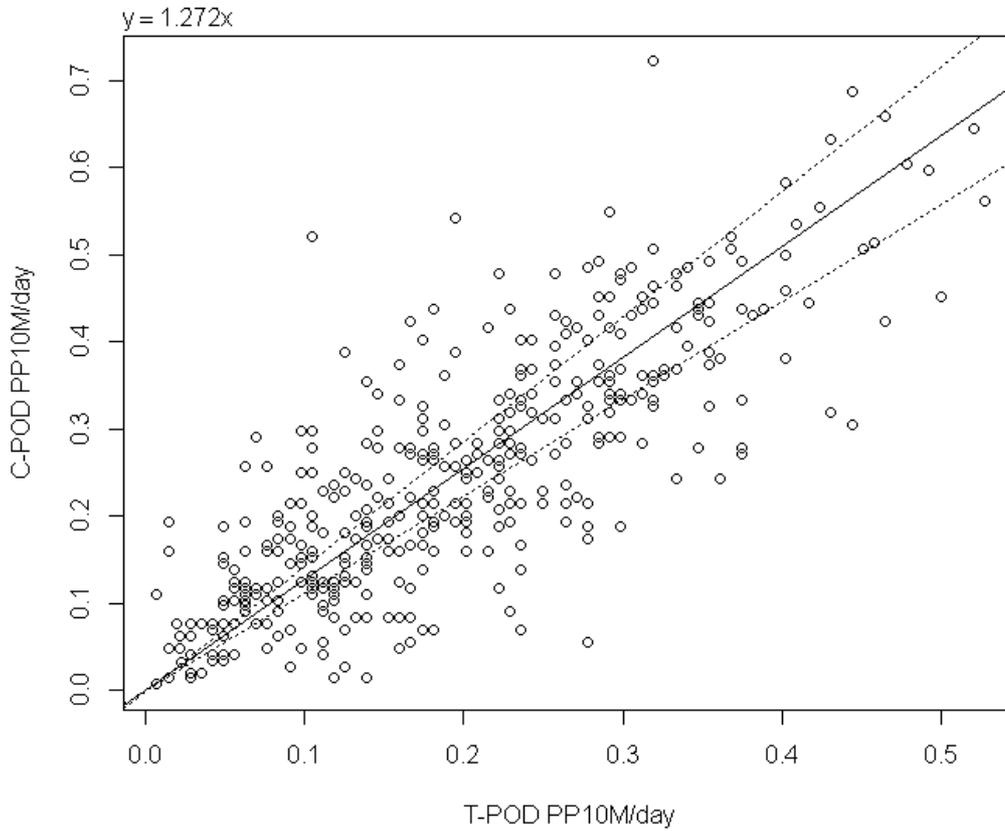
Fig. 8-5: LME modeling of C-POD data on T-POD data (PP10M/day) with the reduced dataset (see Tab. 8-4: eight subsets regarding different T-POD/C-POD combinations;  $N_{total} = 400$ : baseline distribution with LME regression line and CI envelope).
