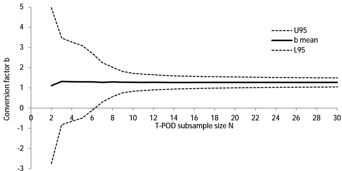
Fig. 8-6: Dependence of the 95% confidence envelope of conversion factor *b* on subsample size  $N_{sample}$  (envelopes are based on 1,000 permutations of  $N_{sample}$  data randomly drawn from the baseline dataset with  $N_{total} = 400$  pairs of T-POD and C-POD data).
