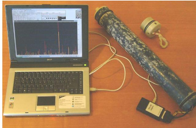
Fig. 2-18: T-POD (version 4) connected with a notebook; this configuration was used during Phase I and Phase II of the project.
