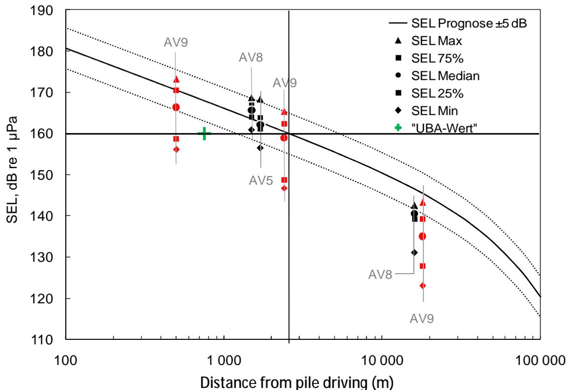
Fig. 2-5: Measured SEL at alpha ventus foundations AV5, AV8, and AV9, as well as predicted curves (after Betke & Matuschek 2011). At AV9 pile driving was conducted with and without noise mitigation system, causing higher SEL variability.
