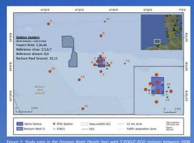
and 2013 (12 positions at a time: red circles: final positions in 2013; st. 12 not analysed here; grey circles: former positions, shifted during the project); blue rectangle: OWF alpha ventus (built in 2009); green grey area: OWF Borkum West III (built in 2011/2012).
