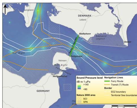
Fig. 2: An example of a noise map generated by Quonops giving a snapshot of the underwater soundscape at 22:00h on 01-12-2021.
