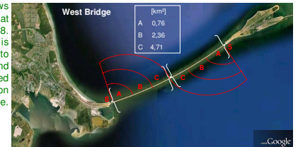
Fig. Map shows scan areas at Positions 5 and 8. Each scan area is divided into sections A, B, and C. Area covered with each section see inset table.
