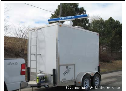
The Canadian Wildlife Service's mobile laboratory for the study of avian migrations.
